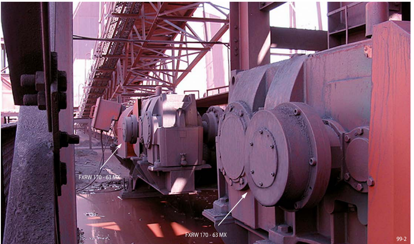
Iron ore conveyor plant in South Africa driven by three gear reducers with RINGSPANN backstops FXRW 170-63 MX.
